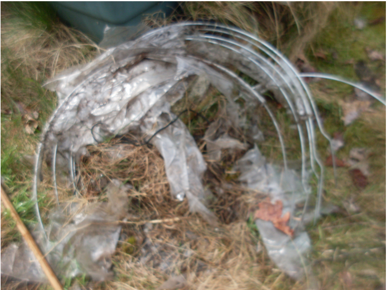
Product corrosion after 3 Year of use (cold frame tunnel film )
